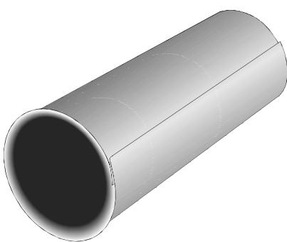
Sleeves are used, along with a mandrel, to coldwork a hole. Made from full hard stainless steel with a baked, dry-film lubricant on the inside surface, they prevent the mandrel from sticking to the hole being coldworked and can only be used once.
